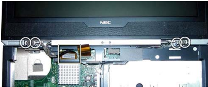
Fig. 21 Removing LCD connector and hinge screws
